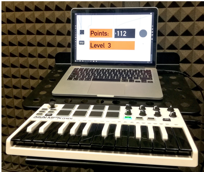
Figure 3.4: The interface of the system: a computer running the software connected via USB to a MIDI keyboard with drum pads.
