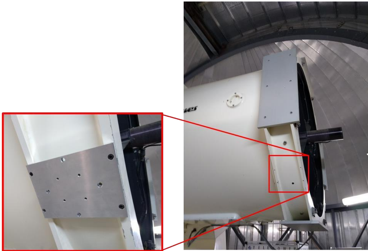
Figure 5-29. Integration of uplink beacon mechanical interface on the telescope tube.
