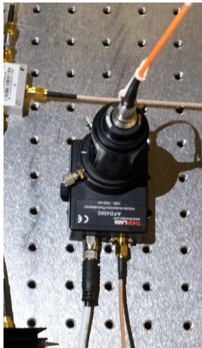
Figure 5-16: MM fiber coupled to optical assembly that focuses the received light into APD receiver sensor.
