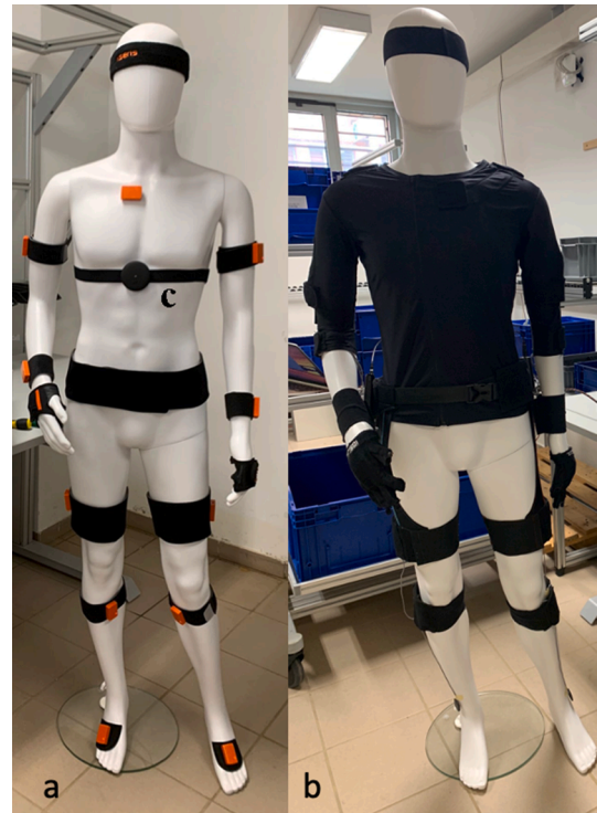
Fig. 2. MOCAP suits used in the laboratory tests: (a) Mtw Awinda, (b) G4 MOCAPSUIT, and (c) the Aidlab activity tracker.
