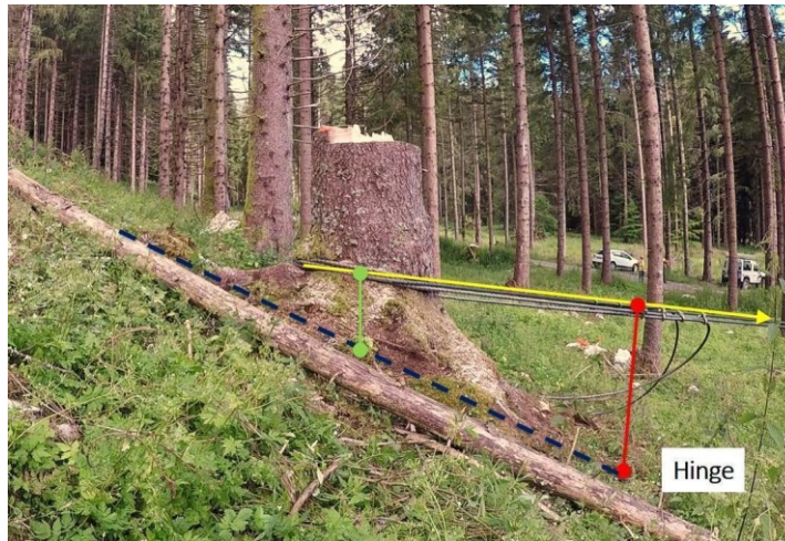
Figure 20. Pulling test of the Stump S1.
