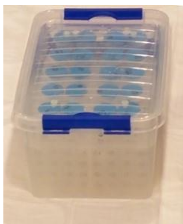
Fig. 1. Water phantom containing 20 tubes filled with MnCl 2 solutions.
