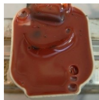
Figure 31: Bubbles on the insulating layer
