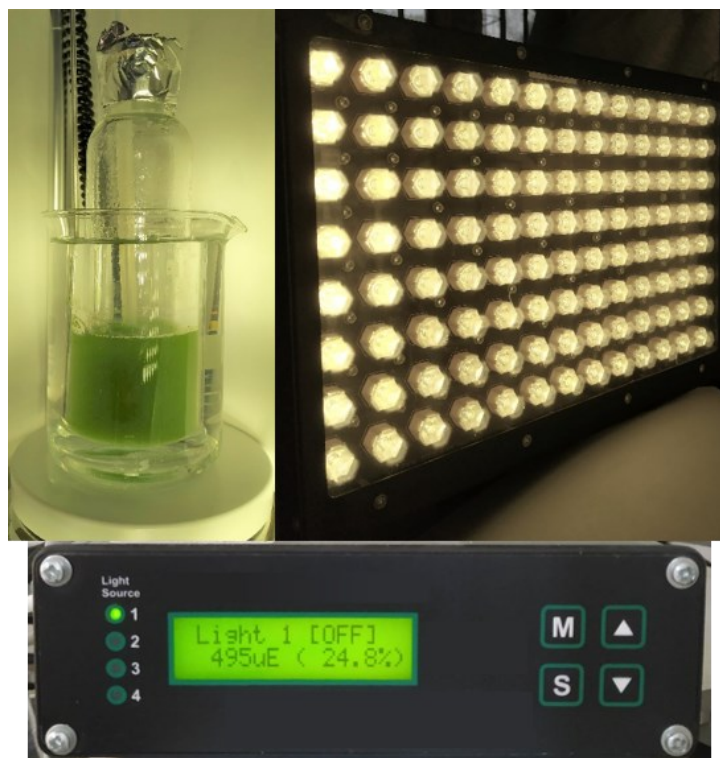
Figure 3.3. Experimental set-up: batch photobioreactor, LED lamp, LED controller
