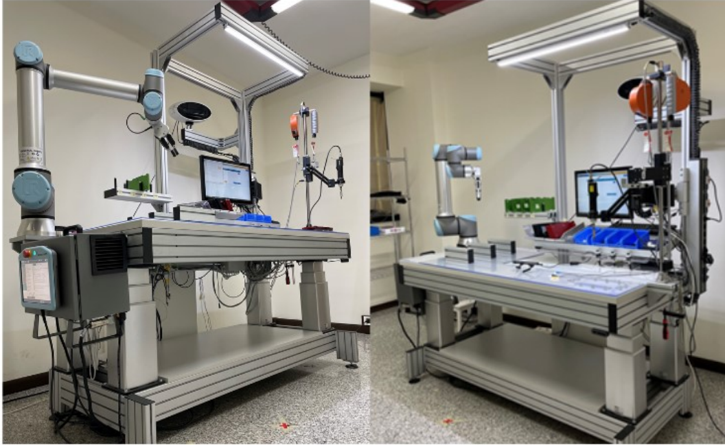
FIGURE 1.1: The robotic arm UR10e and its workstation
