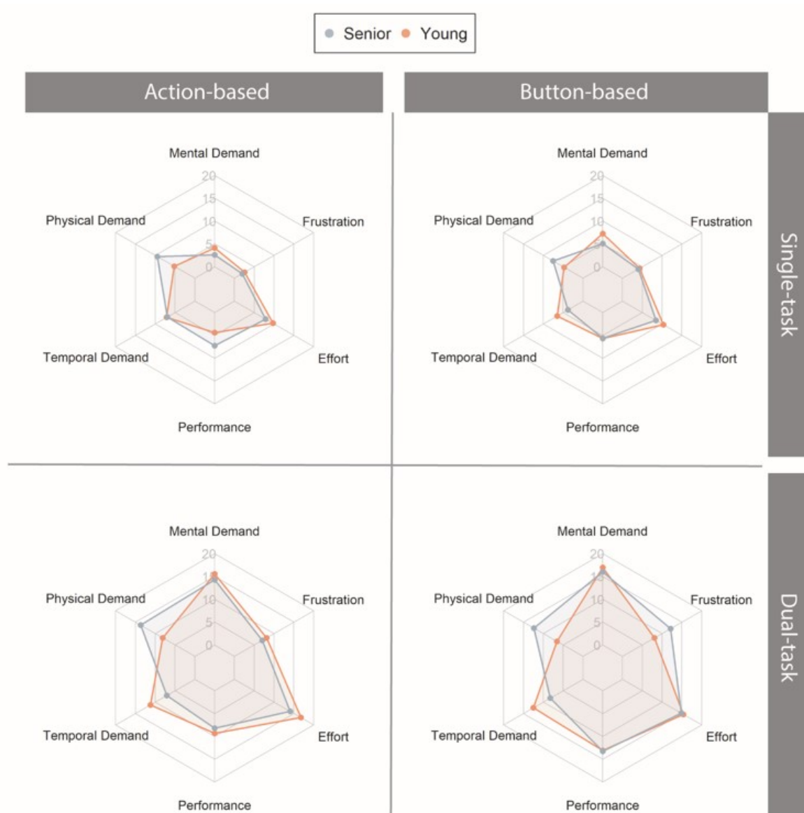
FIGURE 9.9: NASA-TLX questionnaire in young (orange) and senior users (grey) as reported after single- and dual-task executed both via action- and button-based control systems. Results are reported considering the response range of 1-20.
