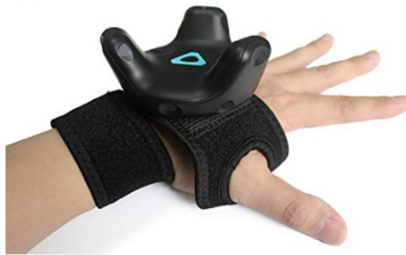
FIGURE 10.1: The VR body tracker applied on the participants' right wrist through the dedicated wristband. Picture from https://www.amazon.de/-/en/dp/B07P93TSDK
