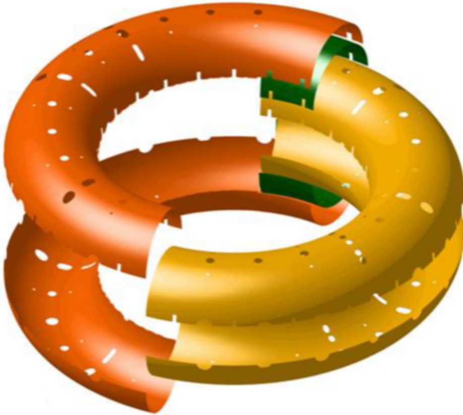
Figure 2.17: Exploded view of the RFX-mod copper shell.
