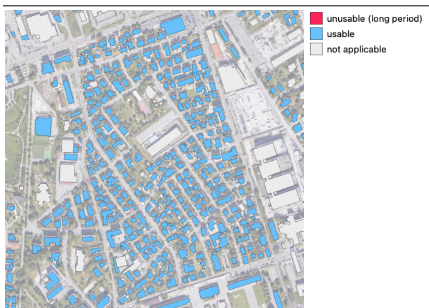
Figure 6.29 - Usability of buildings for a time window of 50 years in Pordenone northern area
