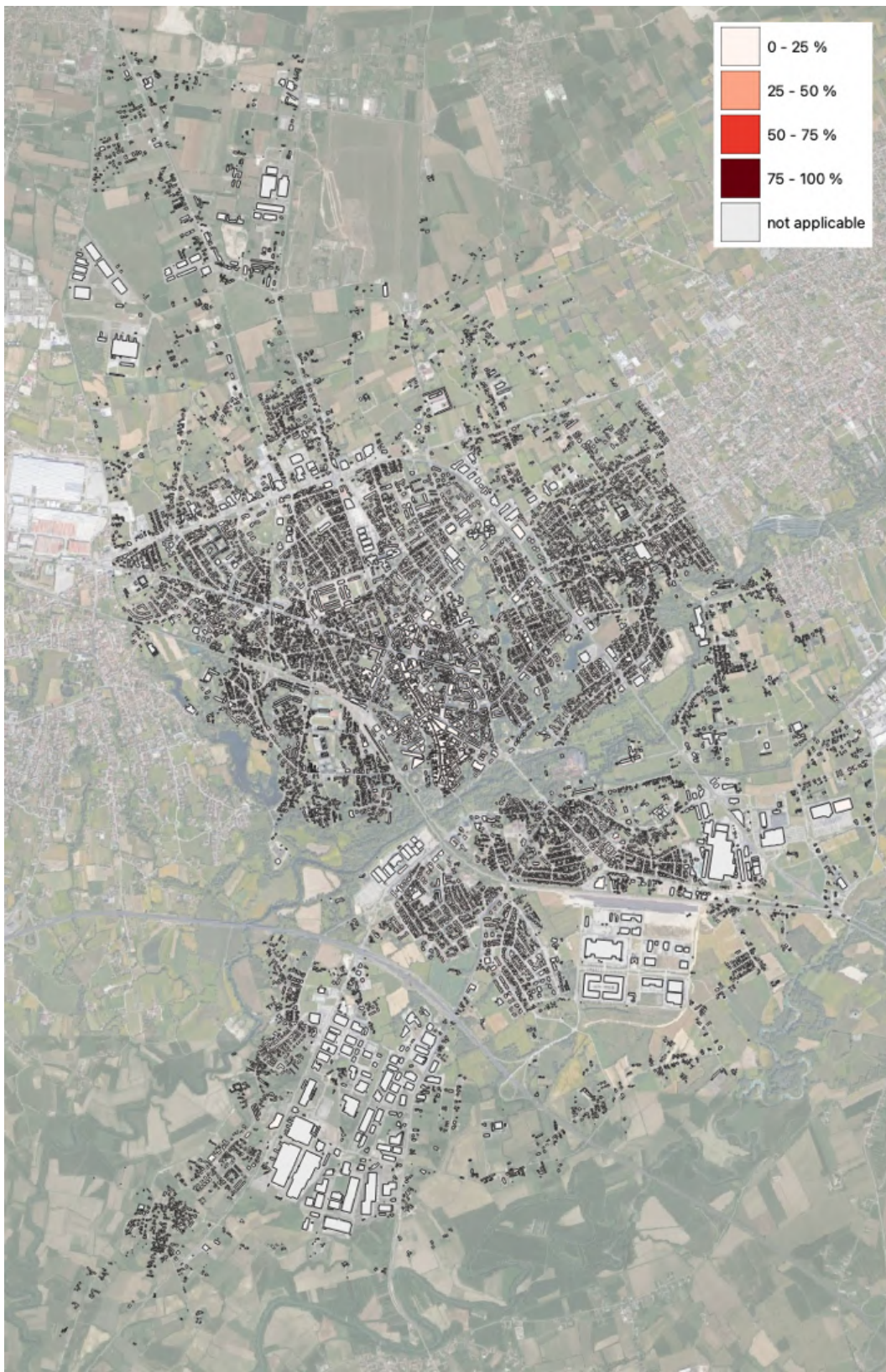
Figure 6.5 - Damage maps DS1, DS3, and DS5 for T_r = 475 years in the Municipality of Pordenone
