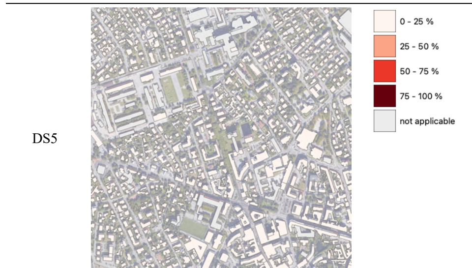
Figure 6.1 - Damage maps DS1, DS3, and DS5 for Tr = 475 years in Pordenone city center
