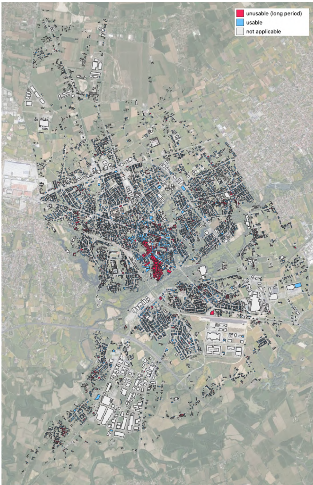
Figure 6.21 - Usability of buildings for T_r = 475 years in the Municipality of Pordenone
