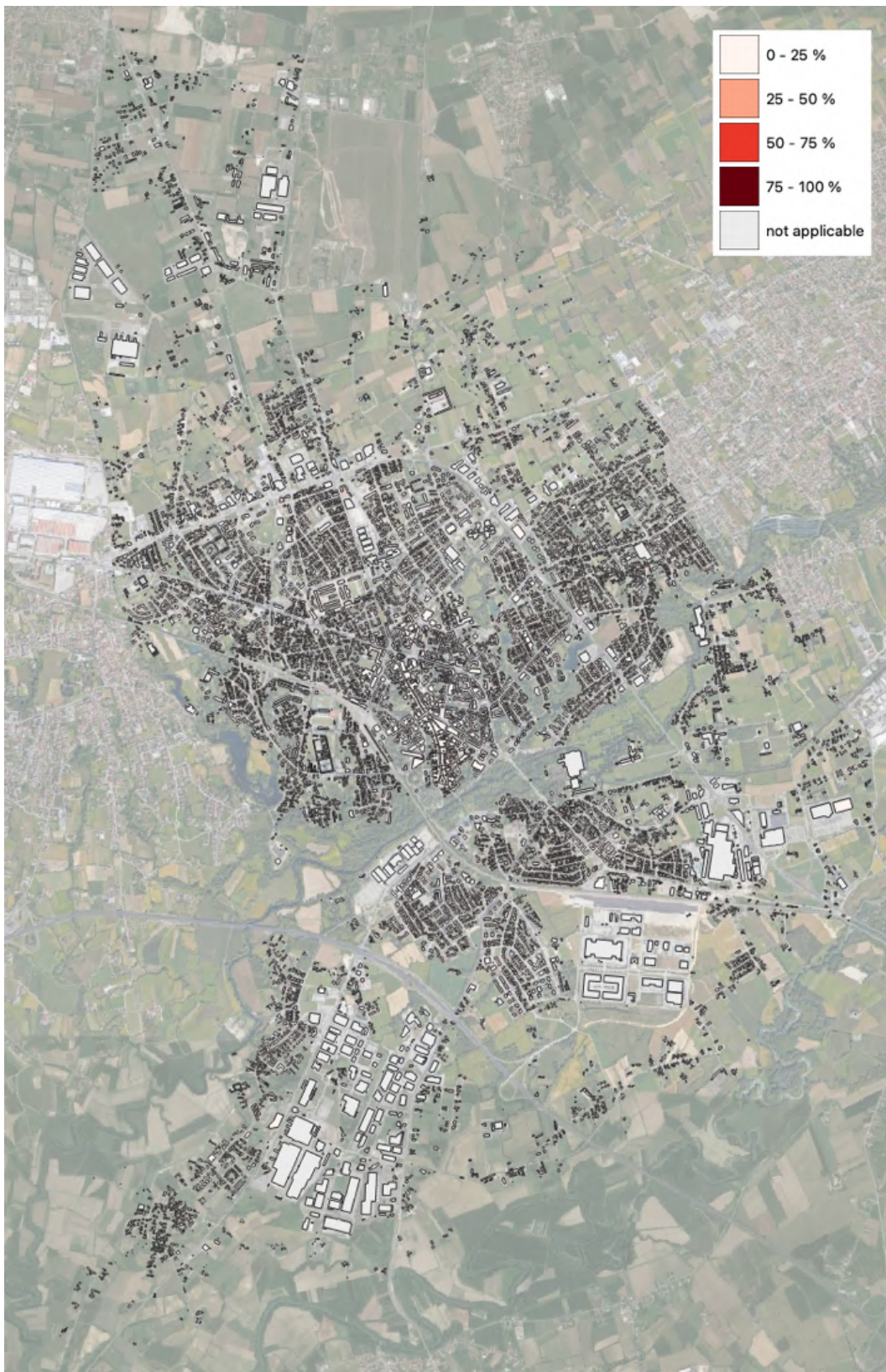
Figure 6.11 - Damage maps DS1, DS3, and DS5 for a time window of 50 years in the Municipality of Pordenone
