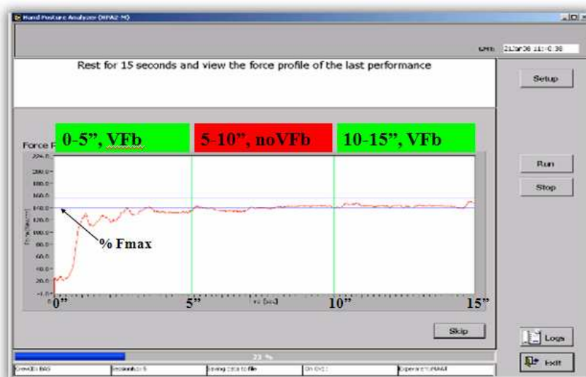
Fig. 3 PGD software display. The three phases of the pull effort can be clearly seen, together with their duration and the line which is offered as a reference to control pulling strength. F_{max} is the force developed in MVC, maximal voluntary contraction, Vfb, period with visual feedback, noVfb, period without visual feedback, REST, rest pause period
