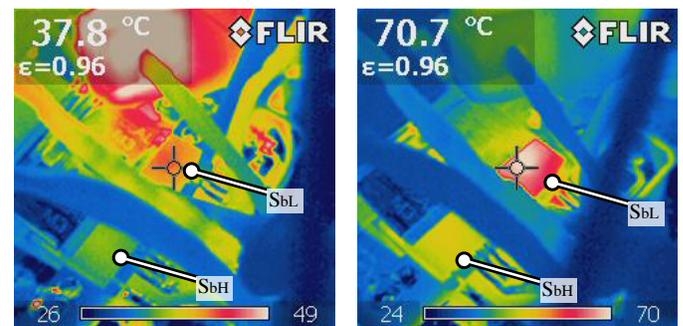
Fig. 15. Thermography of  $S_{bH}$ - $S_{bL}$  at  $V_o = 250$  V during (a) ZVS operation at  $\varphi = 0.25$ ,  $P_o = 2.5$  kW, (b) non-ZVS operation at  $S_{bL}$ ,  $\varphi = 0$ ,  $P_o = 1.1$  kW.
