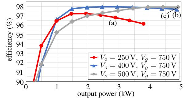
Fig. 17. Measured efficiency at minimum, nominal, and maximum output voltage.
