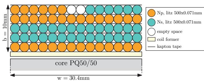
Fig. 11. Winding layout of the designed transformer. Number of turns  $N_p = N_s = 17$ . Each turn is composed of two parallel litz wires  $500 \times 71 \mu\text{m}$  each.
