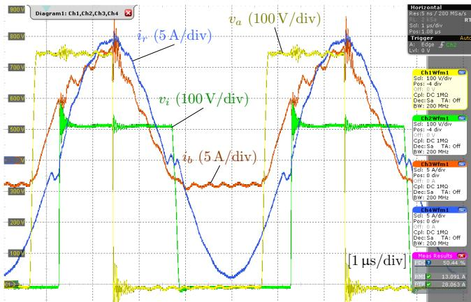
(a) Converter waveforms at  $V_o = 250$  V,  $P_o = 3$  kW. Soft-switching transitions,  $\varphi = 0.2$ .
