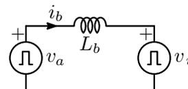
Fig. 4. Equivalent circuit for inductor current analysis.
