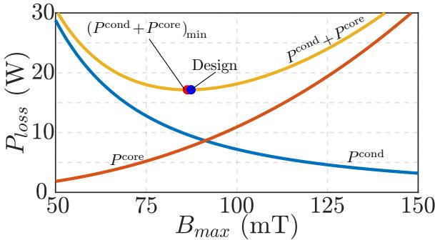
Fig. 10.  $P$ - $B$  plot for transformer design at  $V_o^{\text{nom}} = 400$  V and  $P_o^{\text{nom}} = 5$  kW. The design point is obtained with two parallel litz wires  $500 \times 71 \mu\text{m}$  each and number of turns  $N_p = N_s = 17$ .
