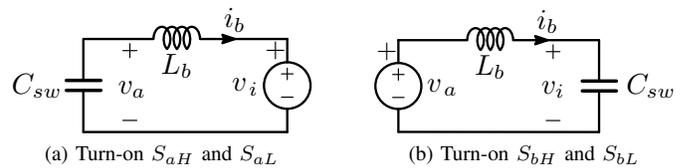
Fig. 5. Equivalent circuits during ZVS transients.
