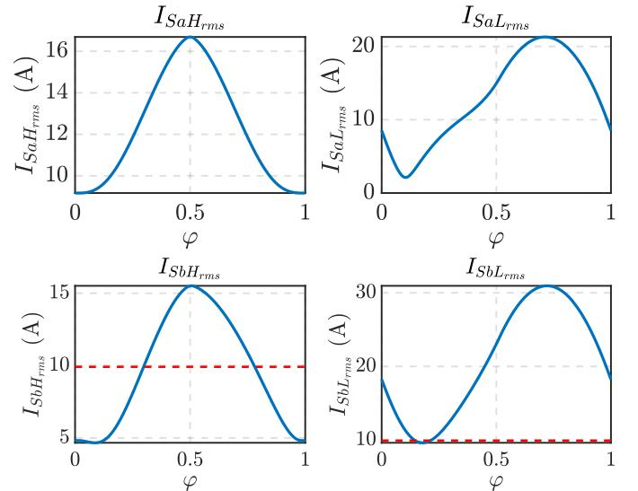
Fig. 8. Switches rms currents at  $V_o = 400V$ ,  $I_o = 12.5A$ . The red-dashed line shows the resonant current component  $i_r$  on the right-leg MOSFETs.
