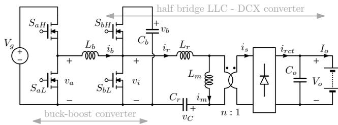
Fig. 2. Two-stage converter with pre-regulation & LLC stage.
