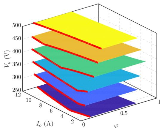
Fig. 6. ZVS regions for the whole output voltage range. Converter parameters are reported in Table III.
