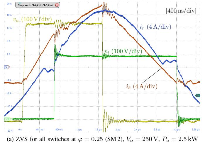
(a) ZVS for all switches at  $\varphi = 0.25$  (SM 2),  $V_o = 250$  V,  $P_o = 2.5$  kW
