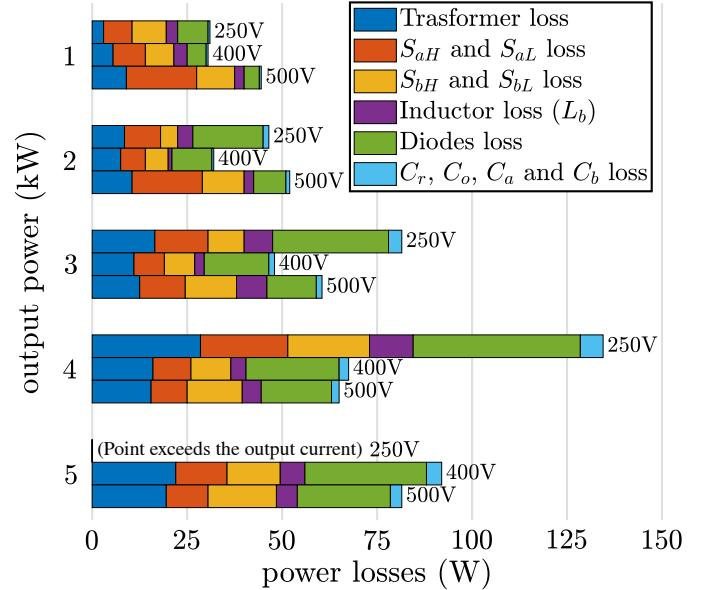
Fig. 18. Loss breakdown at different output power and minimum, nominal, and maximum output voltages.
