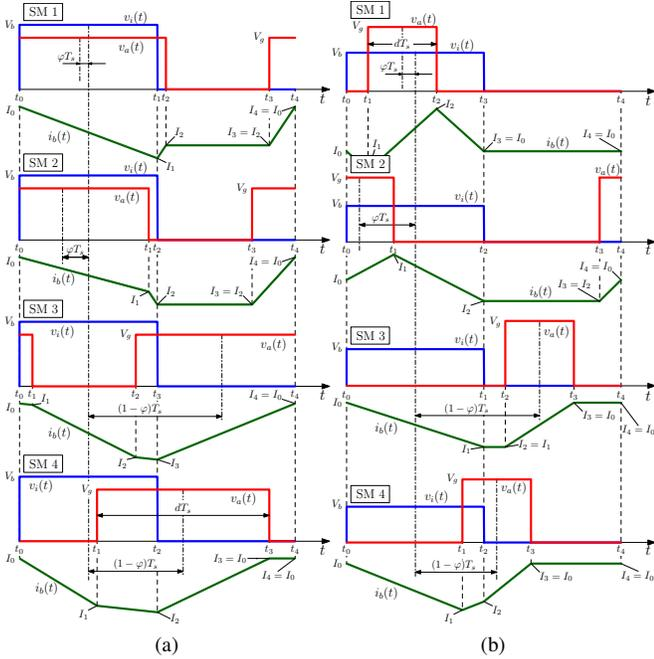
Fig. 3. Main converter waveforms for different phase-shift values considering (a) boost case and (b) buck case. Switching events are marked at time instants  $t_k$  ( $k = 0, \dots, 4$ ), with  $t_0 = 0$  and  $t_4 = T_s$ . The corresponding switching modes are defined analytically in Table II.
