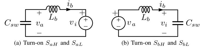
Fig. 5. Equivalent circuits during ZVS transients.
