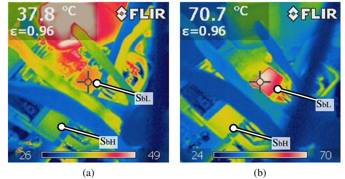
Fig. 15. Thermography of  $S_{bH}$ - $S_{bL}$  at  $V_o = 250$  V during (a) ZVS operation at  $\varphi = 0.25$ ,  $P_o = 2.5$  kW, (b) non-ZVS operation at  $S_{bL}$ ,  $\varphi = 0$ ,  $P_o = 1.1$  kW.
