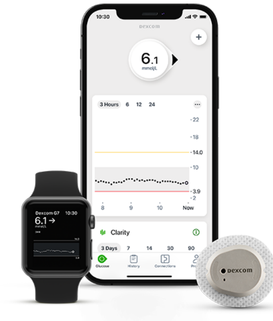
Figure 1.2: Example of CGM device. Dexcom G7 CGM System (Dexcom Inc., San Diego, USA). On the right the CGM sensor and transmitter, and compatible smart devices equipped with Dexcom G7 (mobile app or smartwatch). https://www.dexcom.com
