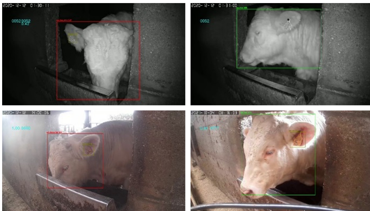
Fig. 2 – Example of system identification results during different moments of the day (during the nighttime in the top pictures; during the daytime in the bottom pictures). It's also shown how the system can discern from “drinking” activity (red square) from the “non-drinking” activity (green square). (For interpretation of the references to colour in this figure legend, the reader is referred to the web version of this article.)
