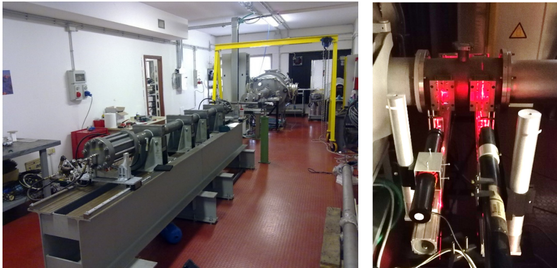
Figure 1. CISAS Hypervelocity Impact Facility with the LGG (left) and laser system for projectile velocity measurement (right).
