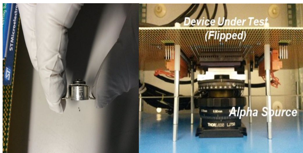
Figure 5-8 Alpha Source and DUT arrangement
