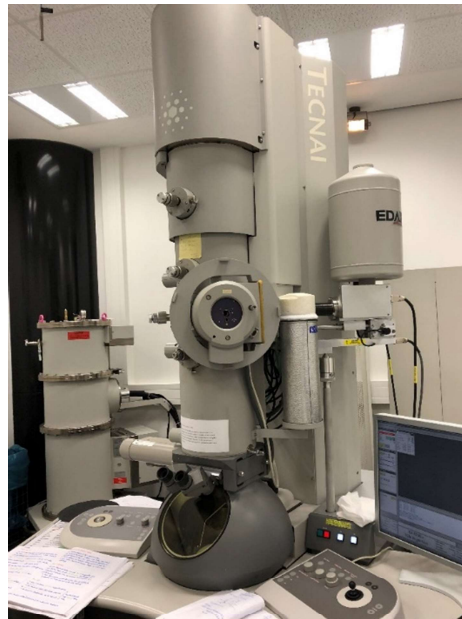
Figure 4.2: FEI TEM TECNAI instrument, ER-C 1 Institute at Forschungszentrum Juelich.
