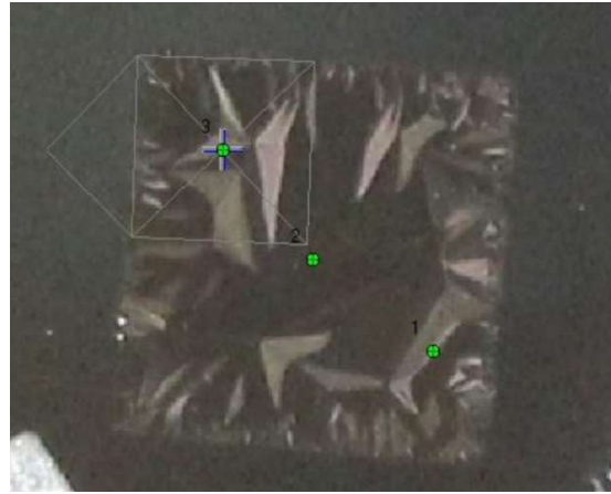
Figure 5.19: XPS analysis was performed in the 3 different shown spots. The measured were performed on the top layer.
