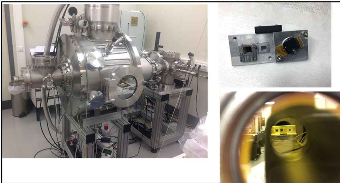
Figure 7.4: Picture of the actual set-up located in ILT institute of Aachen University. In the top image, right side: Scintillator side by side with one of the samples. The holder allows the placement of two samples together with scintillator. In the bottom, right side: Sample placed in the beam pass is shown.
