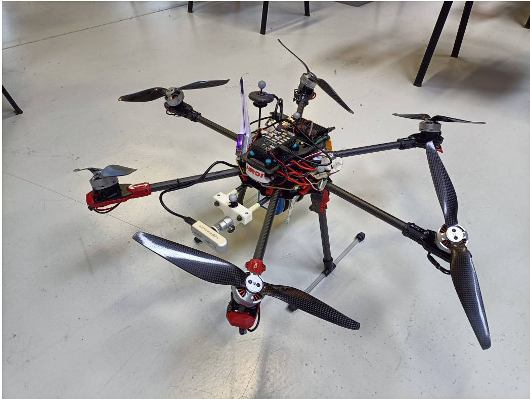
Figure 1.2: Tilted, fully actuated exarotor. Image courtesy of the c-square lab of the Department of Management and Engineering, University of Padova.
