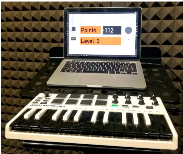
Fig. 1 The interface of the system: a computer running the software connected via USB to a MIDI keyboard with drum pads
