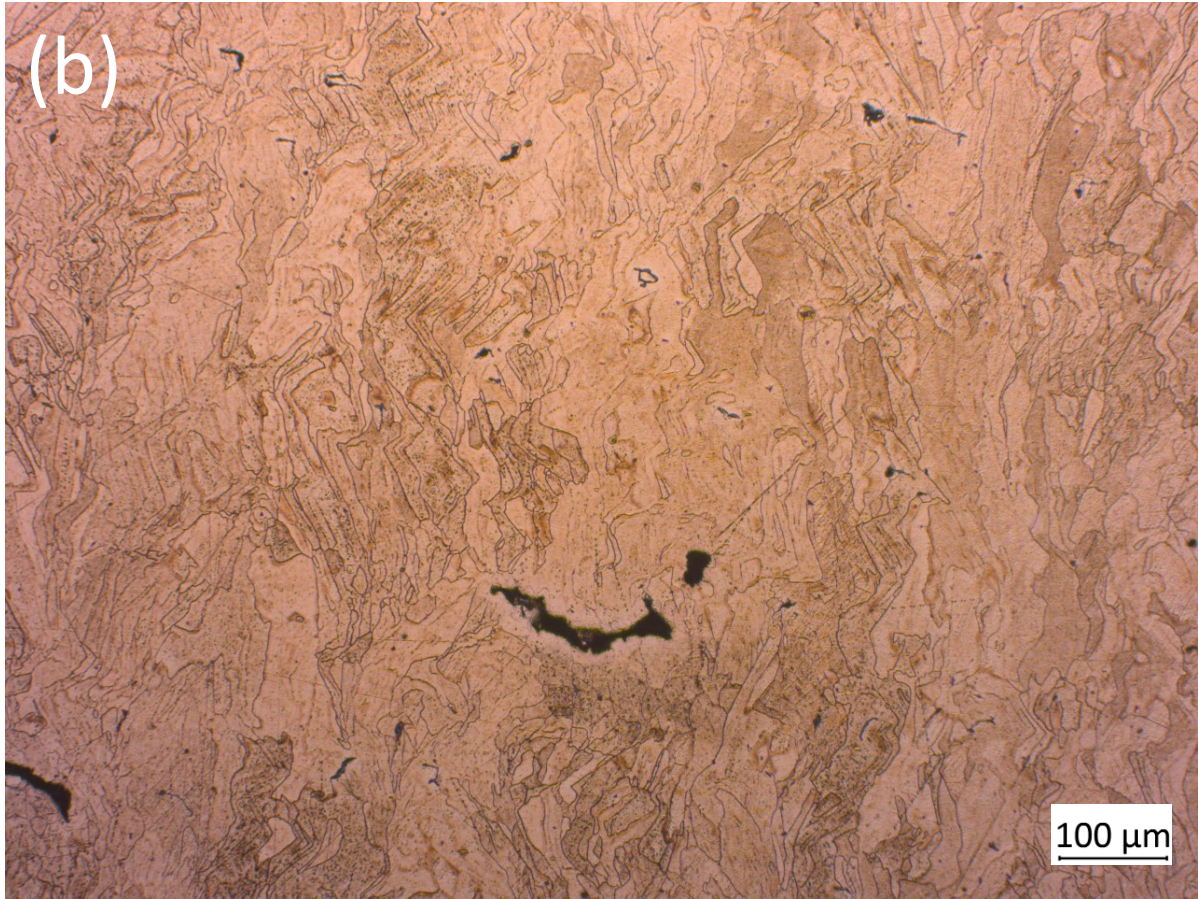
Figure 5.7 Microstructural analyses of XZ section of (a) DAH sample and (b) SA+AH sample.
