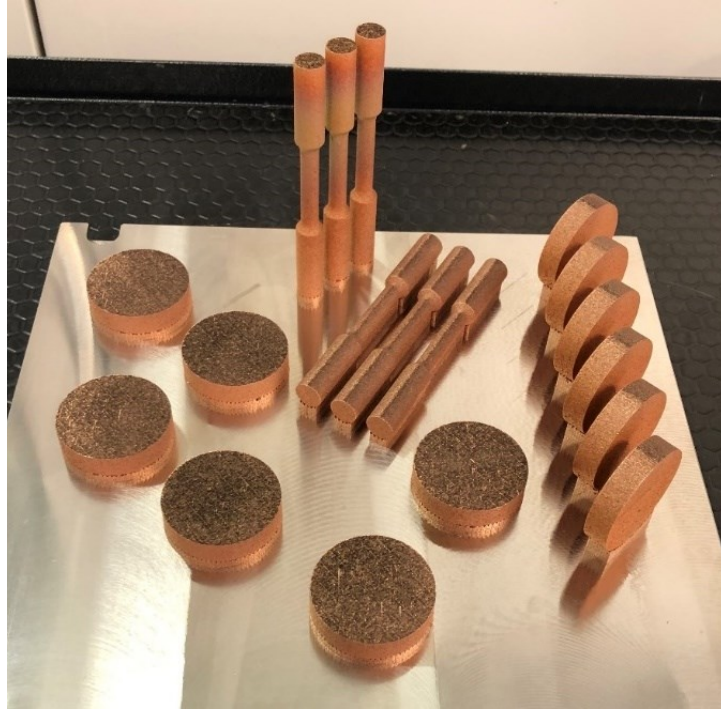
Figure 2.2 Thermal conductivity and tensile specimens manufactured in horizontal and vertical directions.
