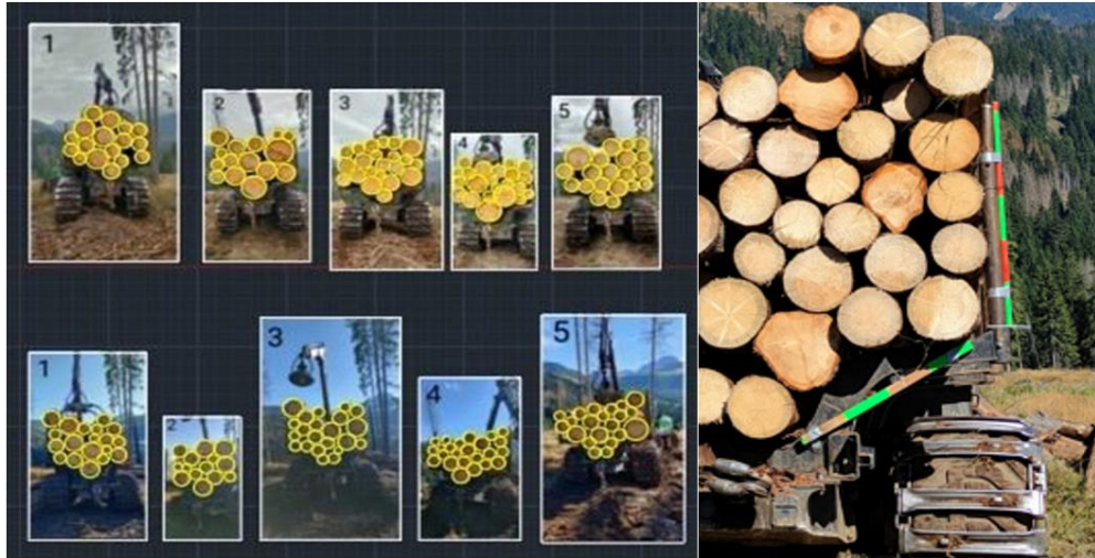
Figure 4.2. Diameter measurements for volume estimation performed with AutoCAD (right) and scale poles for calibration of the volume estimations (left).
