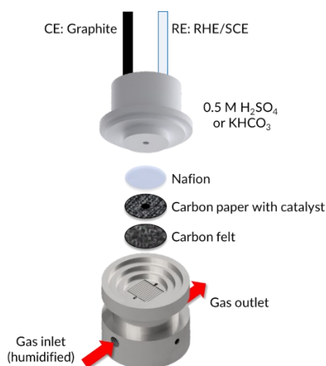
Figure 2.28. Scheme of the cell in all its component
