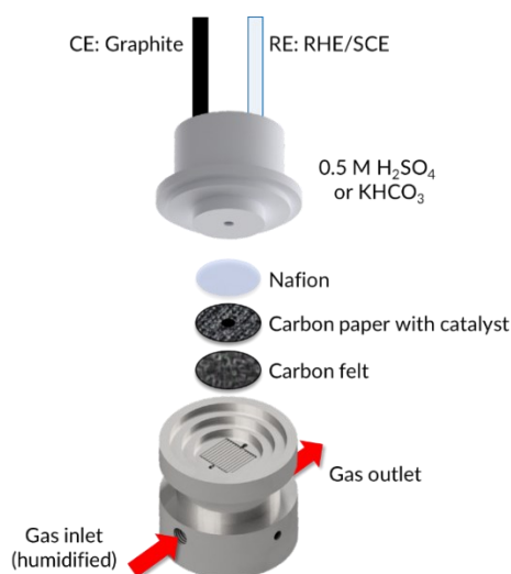
Figure 8.2. Scheme of the cell in all its component.
