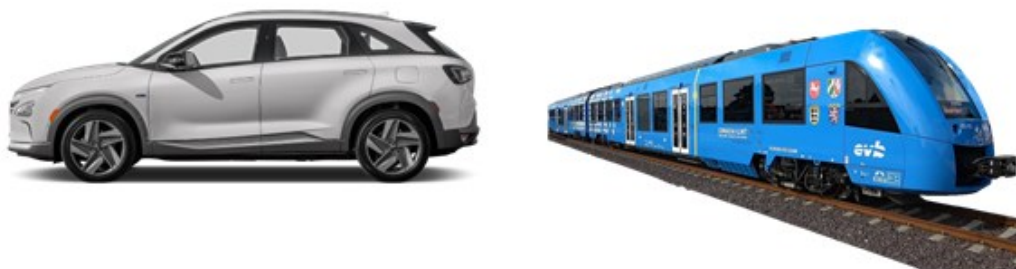
Figure 1.2. Hyundai Nexo on the left and the Coradia iLint on the right, two vehicles powered by fuel cells
