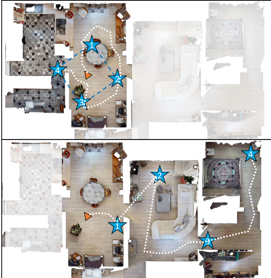
Figure 4.4: Visualizing exploration strategies. ( Top ) shows a Stubborn strategy which selects one of four corners of a local map in a clockwise direction. ( Bottom ) shows a Random strategy where the agent randomly samples exploration goals. We also employ corresponding variants, particularly, Random w/ threshold and Stubborn w/ threshold that have a step threshold (see Sec. 4.4).
