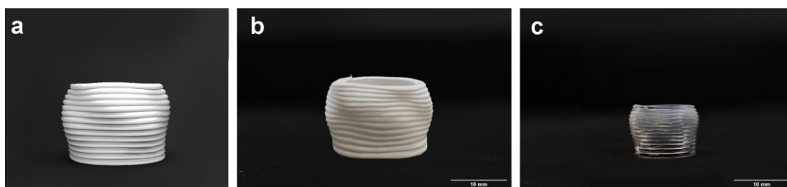
Figure 2.22. Comparison between (a) digital model, (b) printed (green state) and (c) sintered thin wall shape sample.
