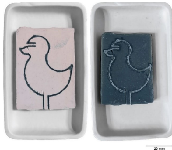
Figure 3.23. tungsten/alumina part example after printing (left) and after thermal treatment under vacuum (right).
