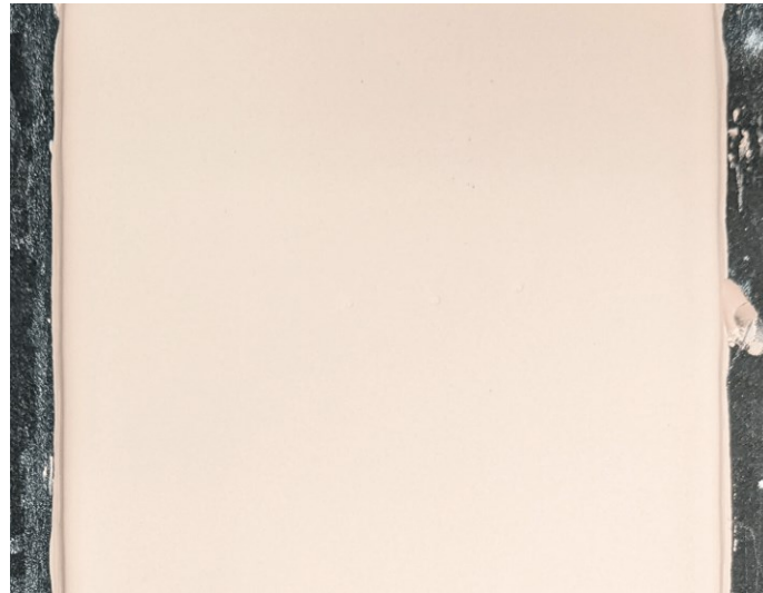
Figure 3.8. Top view of a deposited and dried layer of the HEC based slurry.
