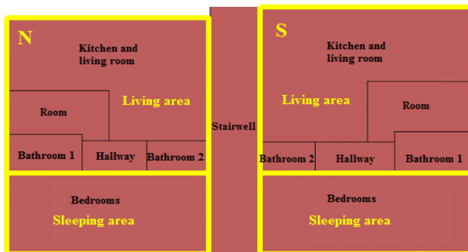
Figure 4.7 Distribution of thermal zones for the apartments.
