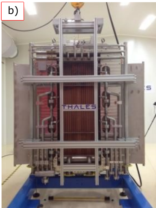
Figure 6.1: a) Dimensions in the accelerator and ED region [43]; b) ED mounted on the SPIDER beam source; c) detail view.
