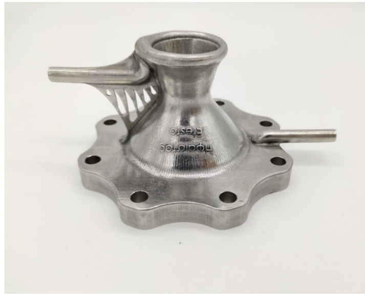
Figure 4. The regeneratively cooled nozzle with integrated mechanical flange to the combustion chamber and inlet and outlet coolant manifolds with associated feeding lines. The nozzle is made in Inconel ® 718 via the laser powder-bed fusion additive manufacturing process.
