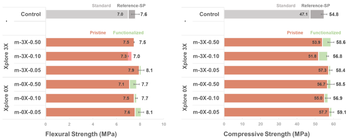
Figure 46: mechanical strengths of mortar samples containing different dosage of GBMs – method B.
