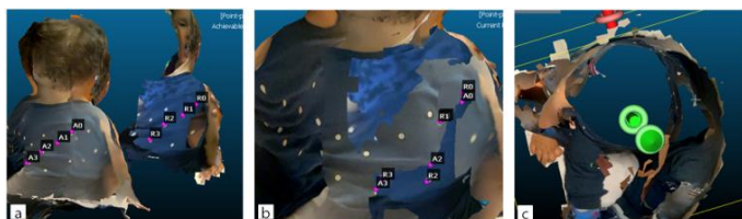
Figure 6. Example of LiDAR scans alignment: a) point selection for alignment; b) alignment; c) top view of alignment.
