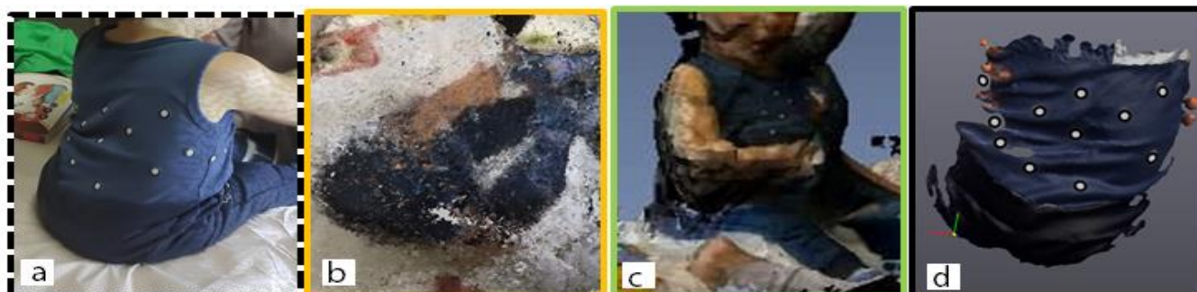
Figure 4. a) Young child torso and detail of scan's output given by b) PH, c) LiDAR and d) SL techniques.
