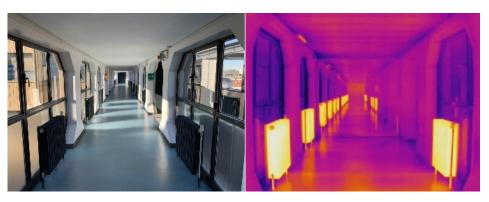
**Figure 7.** Visual (**left**) and thermal (**right**) images of the indoor environment used to test the proposed algorithm. Notice how the thermally distinctive elements on both sides of the corridor are still recognizable in the thermal scene (Figure 8) as well as in the corresponding temperature maps (Figure 9a,b).
