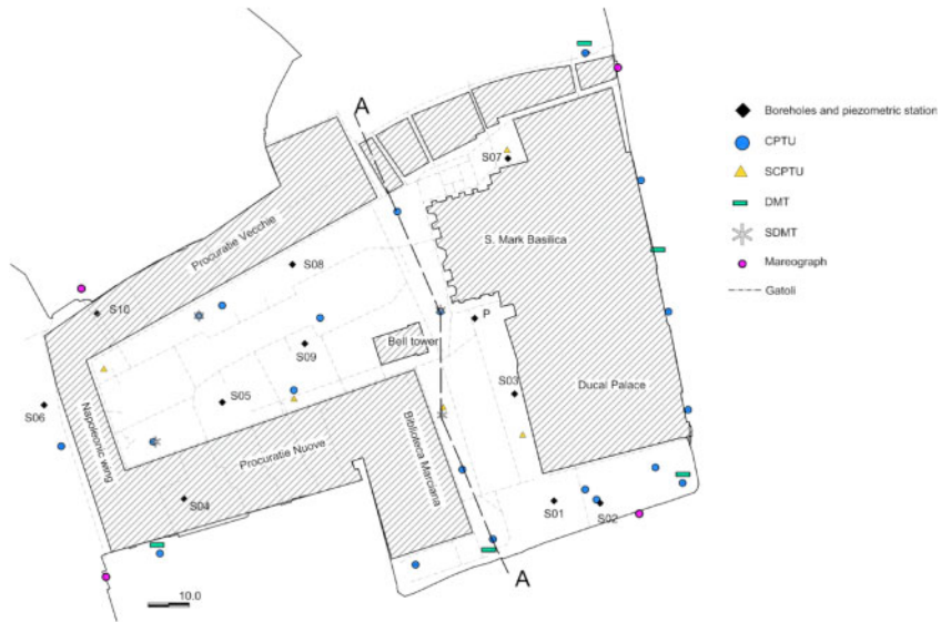
Figure 5. Position of in-situ geotechnical tests (CPTU, SCPTU, DMT, SDMT), boreholes, piezometric stations and old drainage pipes ( gatoli ).
