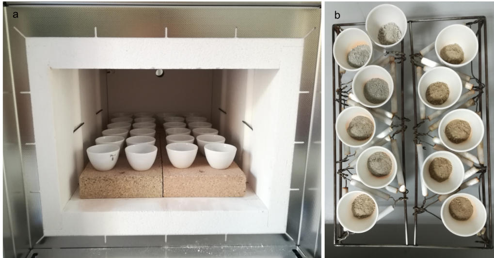
Figure 2.3: Loss-on-ignition samples. Ceramic crucible with ground samples (b) in the muffle furnace (a), where they are combusted at 375 °C for 16 h. The difference in weight, before and after the LOI process, is used to estimate the amount of organic matter, which was combusted, in each sample. Photos: Alice Puppini
