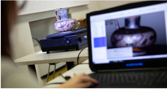
Fig. 2 – Operational image on artefacts from the Marchetti Collection: a structured-light 3D scanning was used to issue a geometric model of micrometric resolution in all its parts; the object was measured with 10 \mu\text{m} accuracy, using an automatic turntable connected to the acquisition software. Photo by Luca Zamparo.
