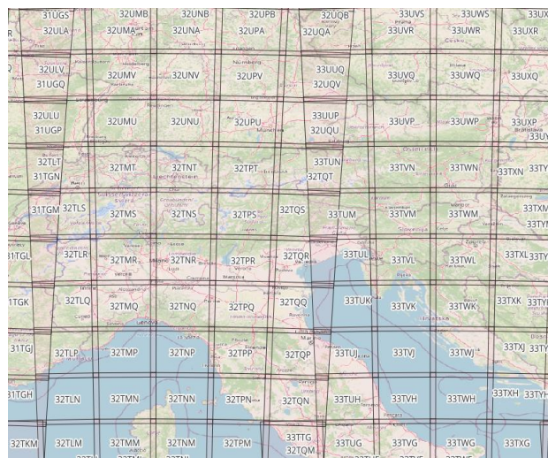
Figure 1. Tiles from Sentinel-2 granules' footprints, with tile coding where the first two digits show the UTM zone and letters the code.
