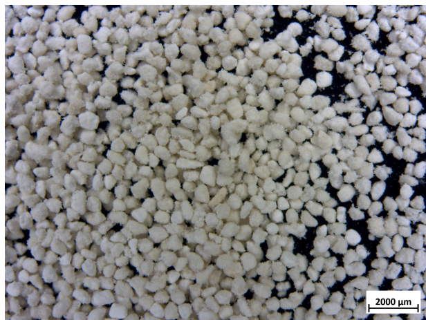
Figure 1.8: Images of the geopolymer granules obtained
