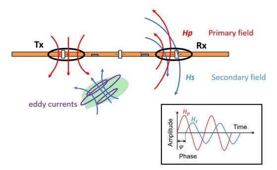
**Figure 2.** Schematic representation of a frequency-domain electromagnetic (FDEM) device, with the corresponding primary and secondary magnetic fields (Hp-Hs) amplitudes and phase lags.
