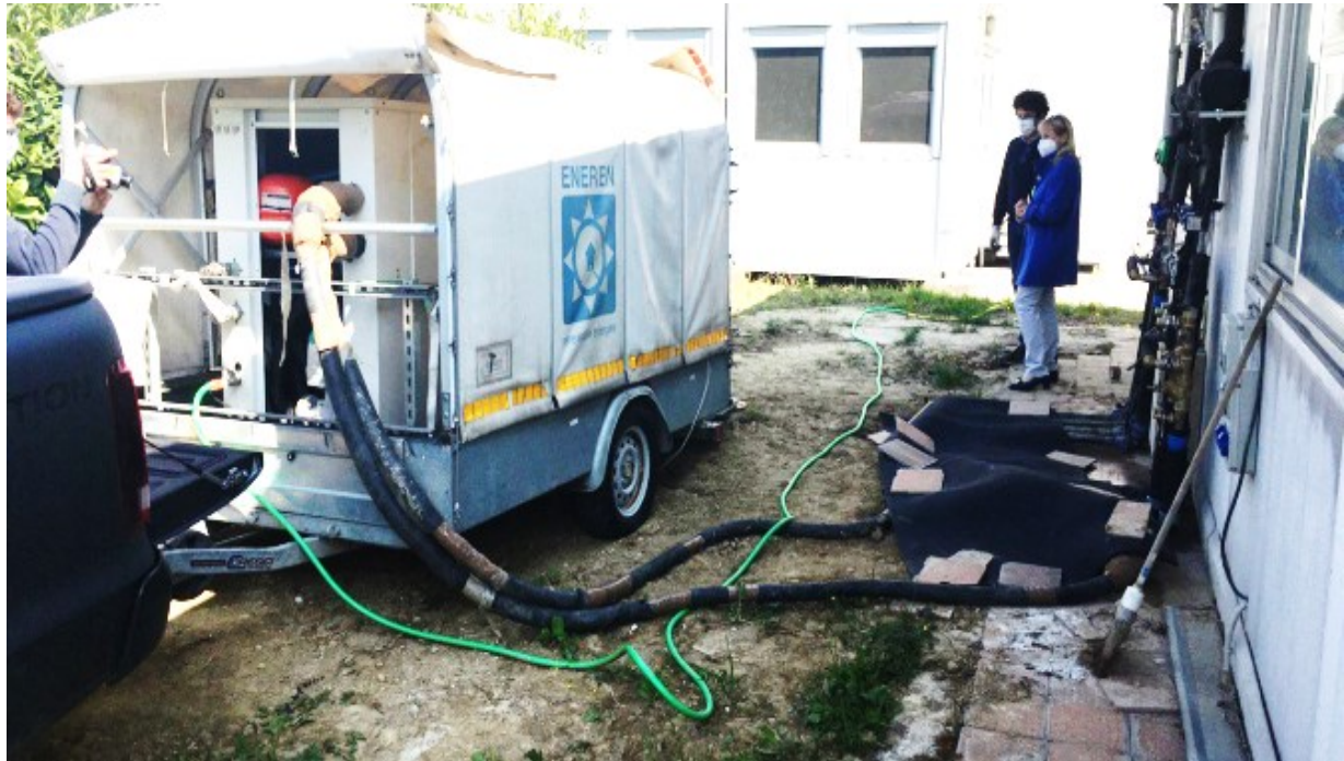
Figure 4: Ground Response Test rig during measurement campaign at the site.
