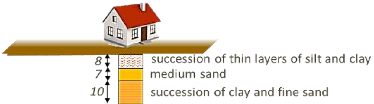
Figure 1: Local stratigraphic diagram. The installed well point GHEs are all deployed within the first 8 meters from ground level.
