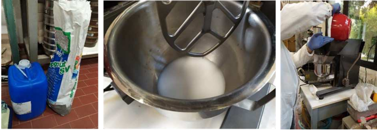
Figure 21: MapegroutSV + IdrocreteS by Mapei (SV) preparation: from left to right the raw material, the additive and the powder mixed to the additive as required by the technical sheet.
