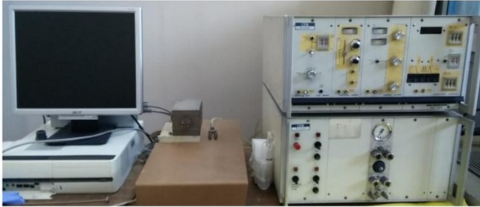
Figure 25: Differential scanning calorimeter with regulation and acquisition system.
