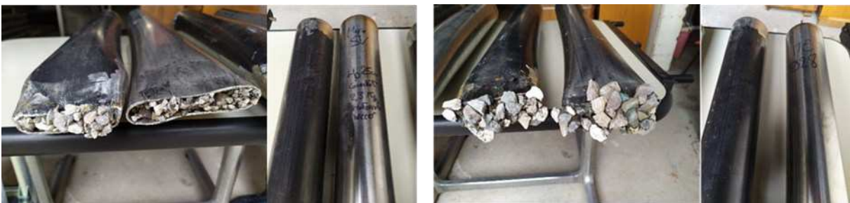
Figure 31: The well points inserted in fine gravel (left) and gravel (right) do not show loss of grouting material, neither SV nor MF928.
