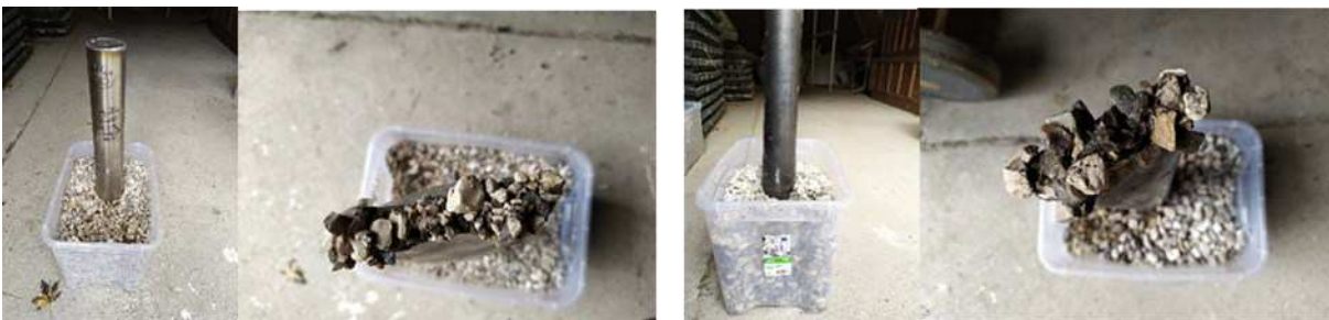
Figure 28: SV after removal: both fine gravel (left) and gravel (right) are completely cemented by the grout where the pipe opening is located. No loss of grout has been detected in the ground.
