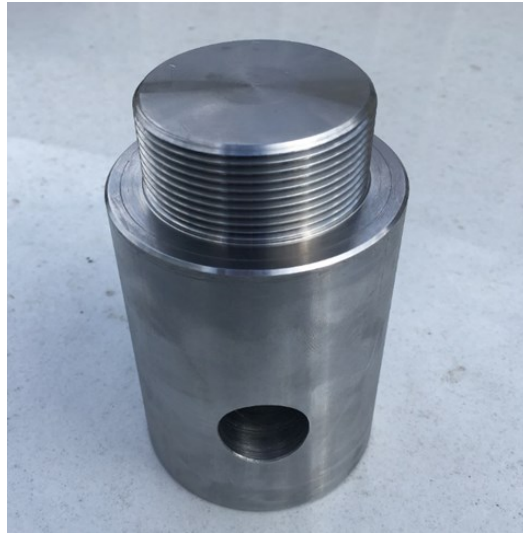
Figure 19: Custom made 2" BSP threaded steel hub.
