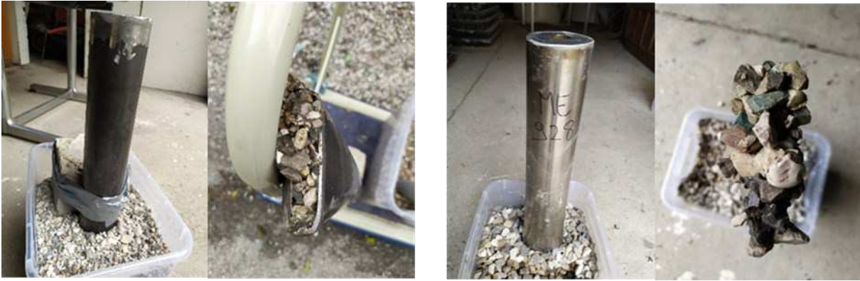
Figure 29: MF928 after removal: both fine gravel (left) and gravel (right) are completely cemented by the grout where the pipe opening is located. No loss of grout has been detected in the ground.
