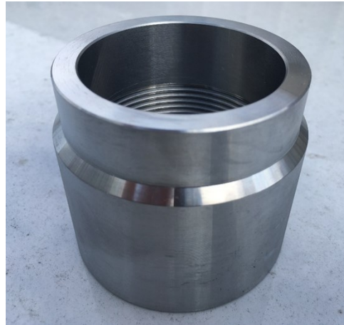
Figure 13: Example of a fitting piece machined in carbon steel alloy. The tapered/recessed section is meant to be inserted into the 3" steel pipe for optimal joint.
