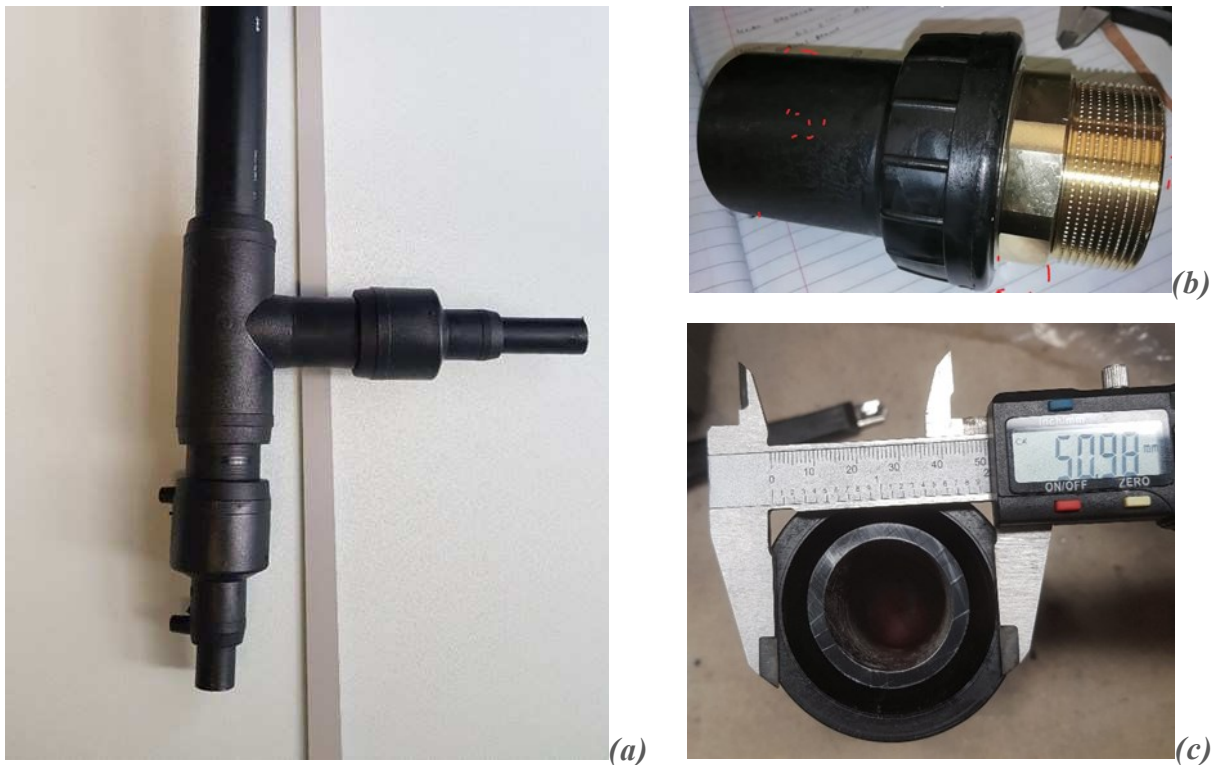
Figure 14: Picture of the prototype of the plastic head assembly (a). Note that the elbow joint was missing in this early design. Detail of the brass 2" male threaded BPS spigot (b). Section of the inner and outer PE tubes constituting the core of head (c).
