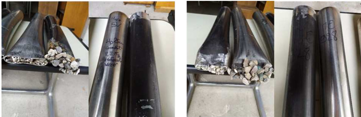
Figure 30: SV (left) and MF928 (right) grouting with different materials (fine gravel and gravel).
