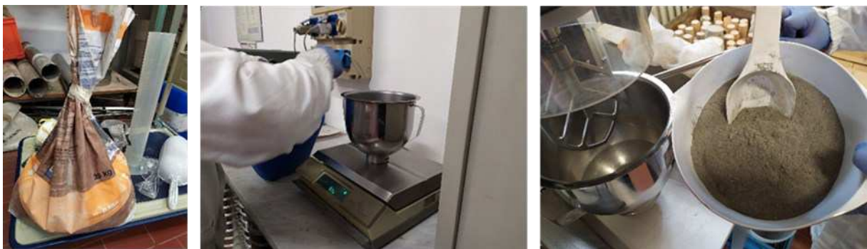
Figure 24: From left to right MF928 raw material, dry powder weighing, mixing with water according to the technical sheet.
