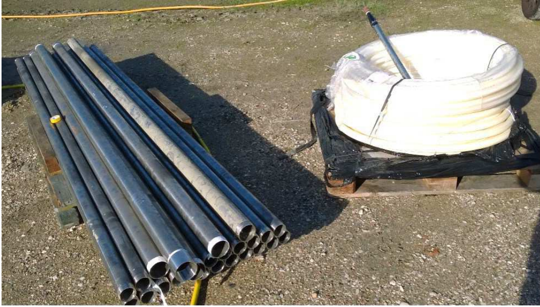
Figure 5: The external coaxial tubes and the internal pipe at the Molinella test site.
