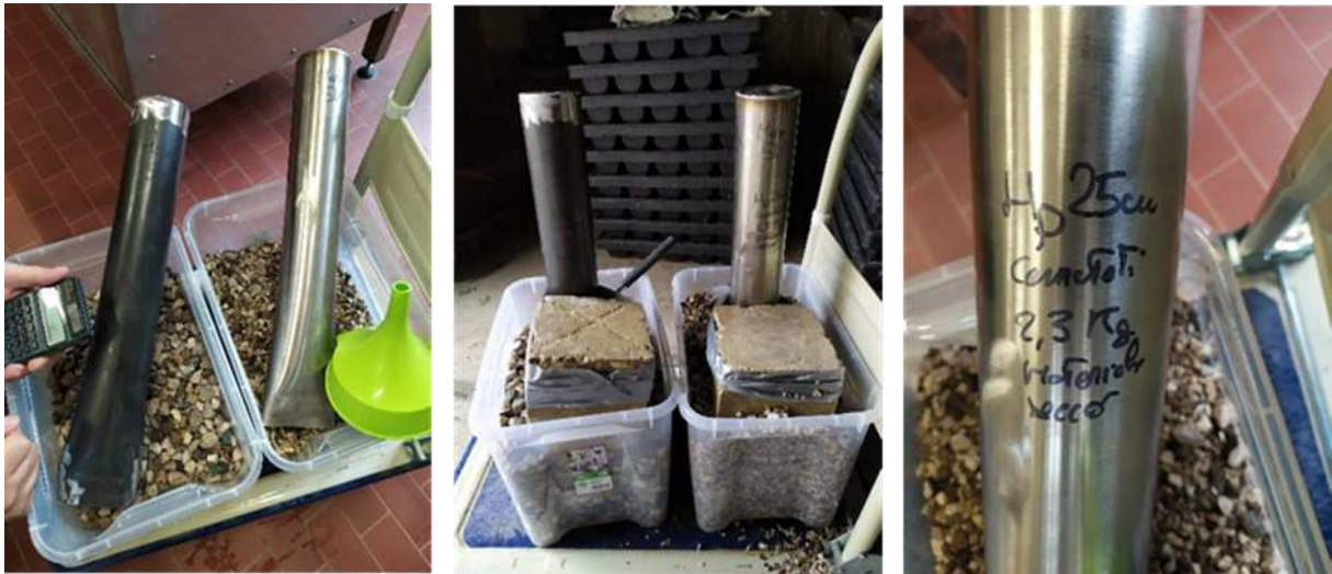
Figure 22: From left to right, preparation to driving the well point into the gravel, securing of the well points and note about the dry material to be used.
