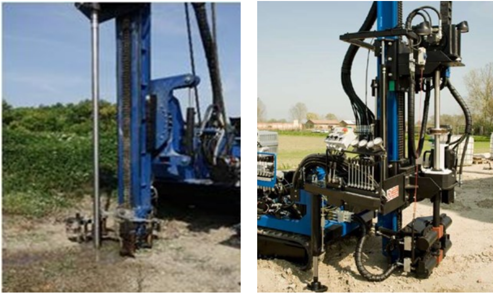
Figure 1: The newly developed drilling machine JOY 4 (left) and the “Vibrasond” machine (right)
