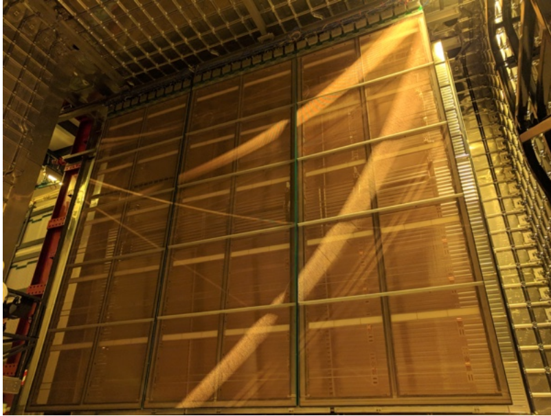
Figure 1: Three APAs in front of the field cage and cryostat wall. The image is originally from [5].
