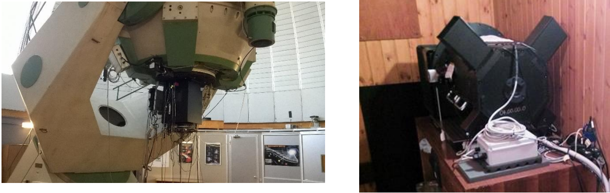
Figure 1. (Left): AquEye+ at the Cassegrain focus of the Copernicus telescope. (Right): rear view of IquEye in the control room of the Galileo telescope with the scientific SPADs and the fiber-optic feed.
