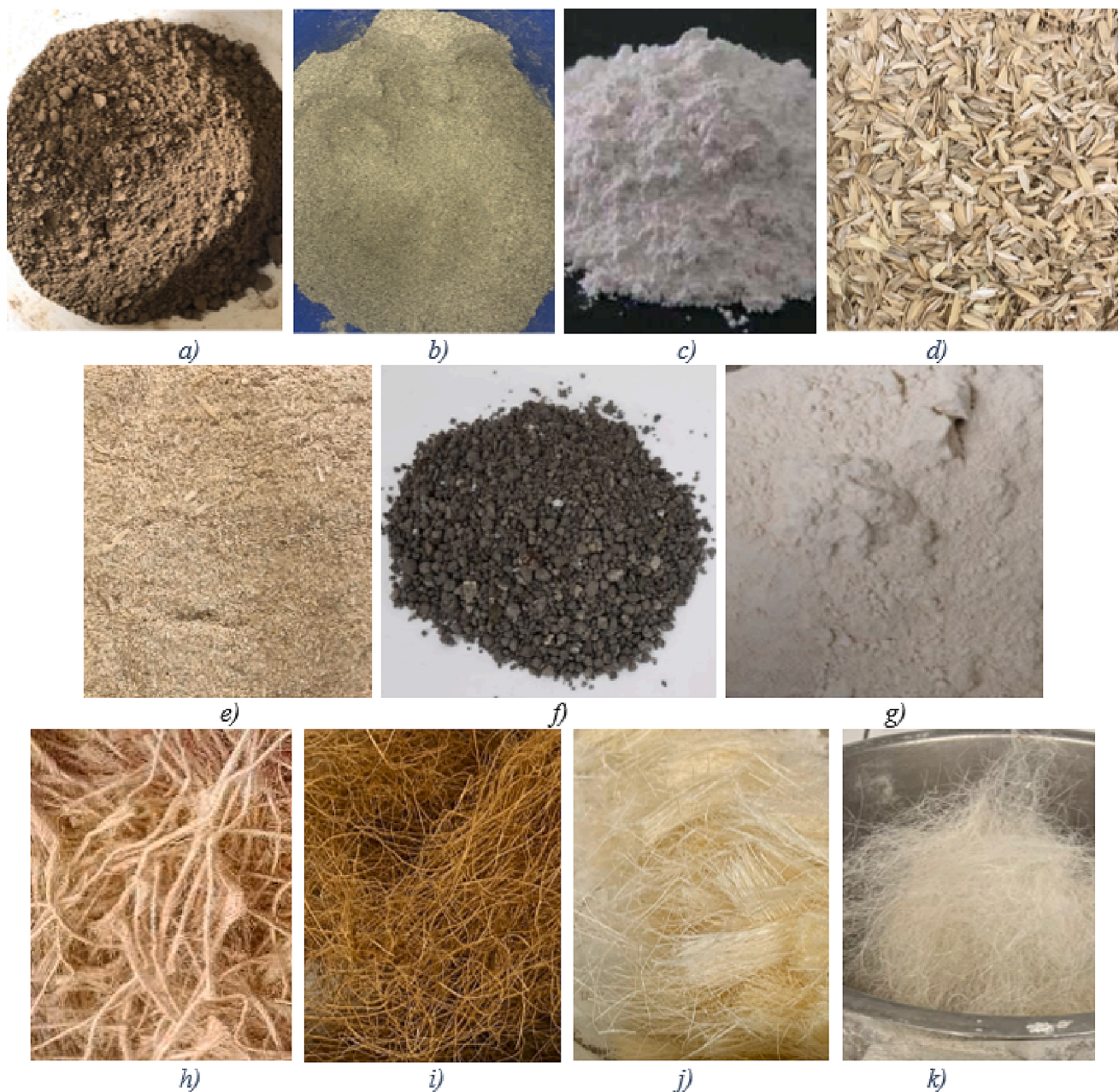
Fig. 2. Materials used for the preliminary 3DP mixes: a) Soil; b) Sand; c) Lime; d) Rice Husk (RH); e) Shredded Rice Husk (SRH); f) Municipal Solid Waste Incinerator Bottom Ash (MSWI BA); g) Marble Dust (MD); h) jute fibers (JF); i) coconut fibers (CF); j) sisal fibers (SF); k) goat hair (GH).
