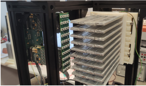
(a) A photo showing a complete module for the x direction. Each SiPM reads a single scintillating finger. A module reads 40 scintillators, all along the same axis, organised as a 4 \times 10 array.
