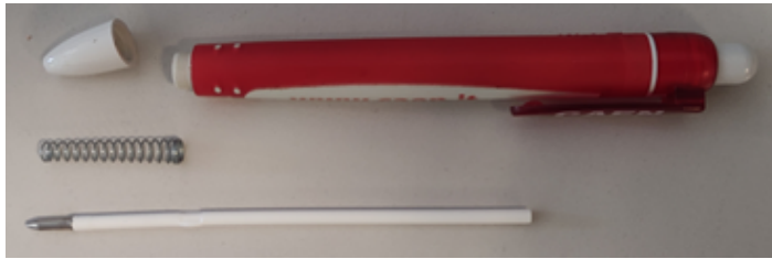
(a) A photo of the ball-tip pen used to try the capability of proton imaging.
