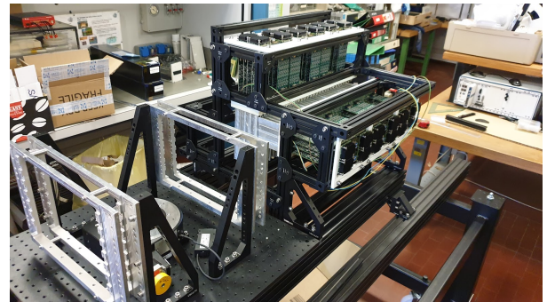
(b) A photo of iMPACT during the final assembly of the prototype. The silicon trackers were not installed yet. The photo was taken in Department of Physics and Astronomy of the University of Padova, GRIT laboratory.
