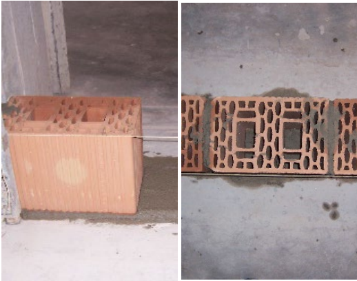
Fig. 2 – Clay hollow brick with horizontal and vertical mortar joints mounted in laboratory
