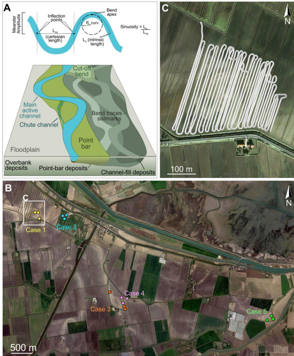
Fig. 6.4. Terminology and methodologies. (A) Morphological, depositional, and morphometric terminology adopted in this paper. (B) The position of the sedimentary cores recovered in the five selected meander bends (Cases 1 to 5) belonging to three different localities (see Fig. 6.1B for the location of this view). (C) The geophysical acquisition: in white dots, the data point acquired in Case 1.
