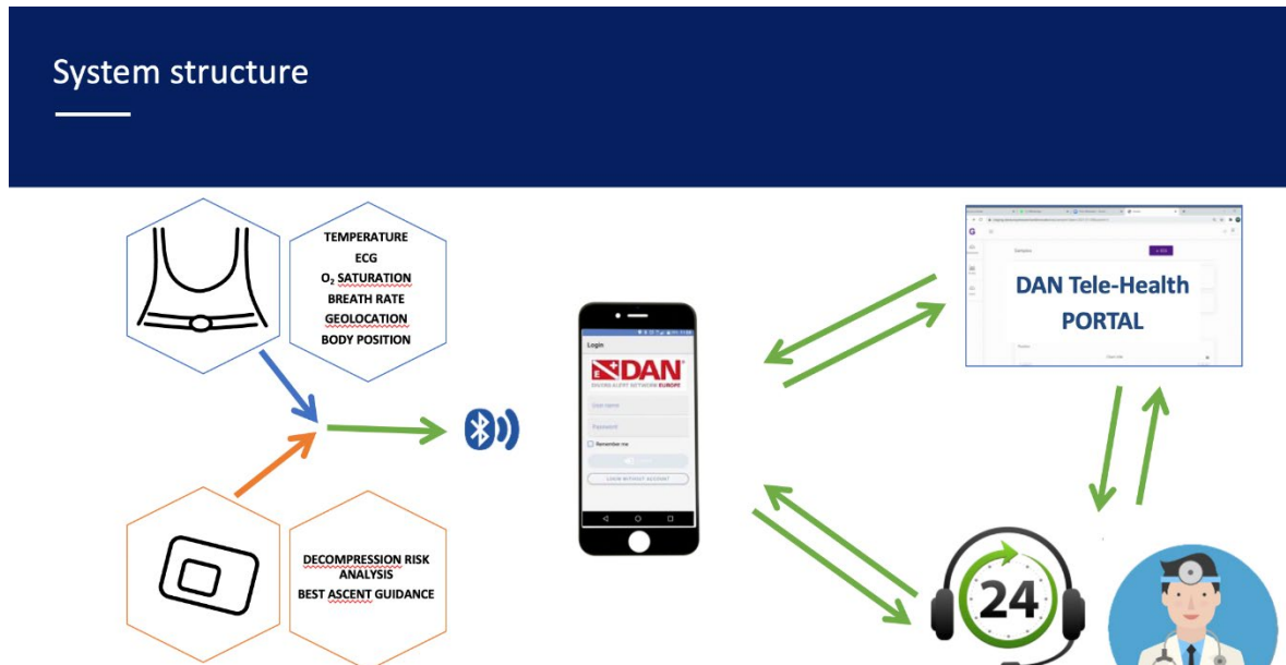
Figure 21 – AVATAR system structure.
