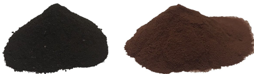
Figure 2. Powder of tannin–furanic polymer (TFP) (left) and mimosa tannin extract (MT) (right).
