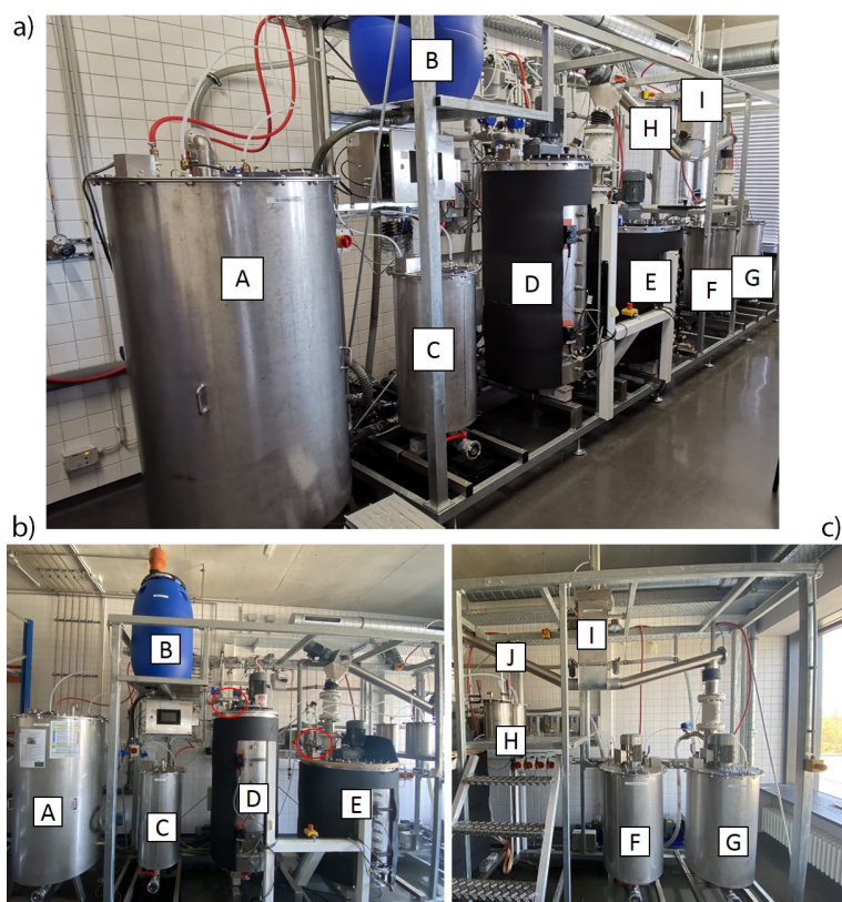
Figure 2. Scaled-down biogas plant in the biogas laboratory of the THI consisting of (A) slurry storage, (B) water tank, (C) fermentation residue tank, (D) bioreactor 1, (E) bioreactor 2, (F) pre-storage tank for liquids, (G) pre-storage tank for mixed substrate, (H) screw conveyor for automatic feeding, (I) pre-storage tank for solids, and (J) the water filter system. (a) Entire biogas plant and details of (b) the left and (c) the right part of the biogas plant. Red cycles indicate the cast housing of the GRP filters.
