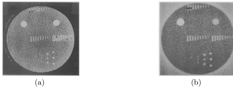
Fig. 20: (a) 320 \times 320 pixels display from the EMI 5005 X-ray CT scanner. (b) Proton CT reconstructions of a 30 cm phantom performed by Hanson in 1979 at Los Alamos Meson Physics Facility (LAMPF). Images from [63]. Note the higher contrast for protons but the better X-ray resolution.
