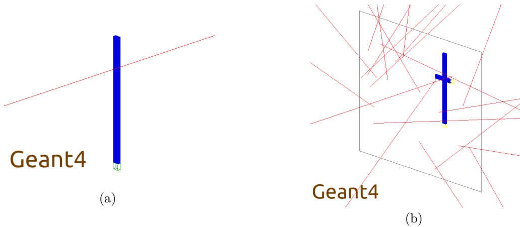
Fig. 67: (a) Rendering of the cosmic rays simulation in the first version, including a single scintillator and a pencil beam. (b) Layout of the second version of the simulation, including two perpendicular scintillators and a planar cosmic rays source [144].
