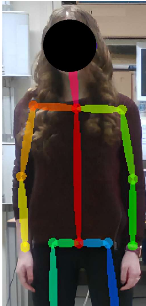
Figure 1. Markerless MoCap example. The colored lines represent the detected body parts.
