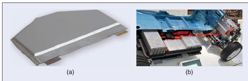
FIGURE 6 – Li-ion cell packages. (a) A hexagonal lithium–polymer cell for underwater vehicles. (Source: https://en.wikipedia.org/wiki/File:Custom_Cells_Itzehoe_GmbH_free_form_factor_battery_for_Unmanned_Underwater_Vehicle_(UUV_AUV).png .) (b) A LIB of a Nissan Leaf, first generation (2009 model: 7.6 V 24 kWh; 2023 models are provided with batteries rated 350 V, 40–62 kWh). (Source: https://en.wikipedia.org/wiki/File:Nissan_Leaf_012.JPG .)
