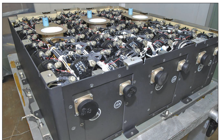
FIGURE 4 – The Hubble battery module assembly with lid removed, showing the Ni-H 2 cells and power isolation switches. (Source: https://en.wikipedia.org/wiki/File:218582main_Batt_FS_img1_lg.jpg .)
