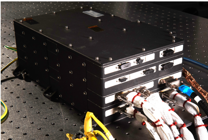
Figure 3.4: Flight model of Main Electronic Unit (MEU). Courtesy of Leonardo S.p.A.
